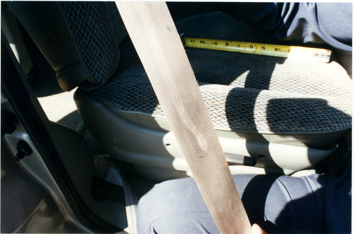
92. View of the fluid spill. Note, this is the reverse side of the webbing.
